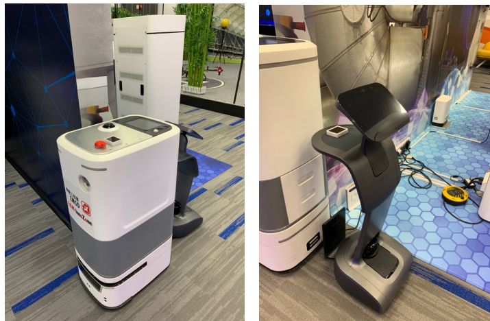
Fig. 14. Two robots on 4/F deployed with luXbeacon
